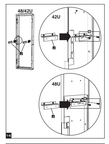
Use two M6 x 12 mm flat-head screws **K** to attach each hinge **1** as shown. **Orient each hinge so that the pin is closer to the outside of the frame than the inside.**
